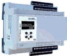
Universal input and output module for KNX IP-only. The device offers 48 digital channels. Each channel can be used as a binary input, binary output or blind output. Input channels can be used to connect buttons. Output channels can directly control signal LEDs, external coupling relays or blind relays. The peripherals (e.g. relays) are supplied by an external power supply (24 V $\overline{=}$ ). The device works using the medium KNX IP and is connected to the KNX installation via LAN/Ethernet.
