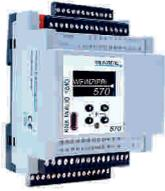
Universal input and output module for building control. The device offers 48 digital channels. Each channel can be used as a binary input, binary output or blind output. Input channels can be used to connect buttons. Output channels can directly control signal LEDs, external coupling relays or blind relays. The peripherals (e.g. relays) are supplied by an external power supply (24 V $\overline{=}$ ).
