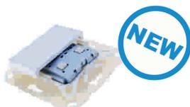
The wireless KNX RF/ENO Push Button Insert 440 *secure* offers support for EnOcean and KNX RF in one device. The device operates in EnOcean mode without configuration (EnOcean Security is activated via a simple push button combination). By configuration with the ETS®, the push button switches to KNX RF mode and offers an optional support of KNX Security.
