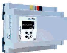
The device combines the central functions of a KNX bus line: bus power supply with bus choke, KNX IP Router and KNX IP Interface with small space requirements. The KNX IP Router in the LineMaster enables the forwarding of telegrams between different lines via a LAN (IP) as a fast backbone. The device also serves as programming interface between a PC and the KNX bus (e.g. for ETS® programming).
