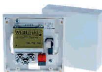
Bidirectional gateway between EnOcean radio and the KNX bus. The device supports encrypted radio communication with security-capable EnOcean devices. Over 100 device profiles (EEP EnOcean Equipment Profiles) allow simple and secure connection of different EnOcean sensors and actuators to KNX installations.
