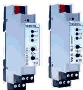
Compact switch actuator with one bi-stable output and 2 binary inputs. Suitable as KNX-compatible replacement for conventional impulse switches (output: lights, input 1: push-button, input 2: L for zero-crossing detection).
