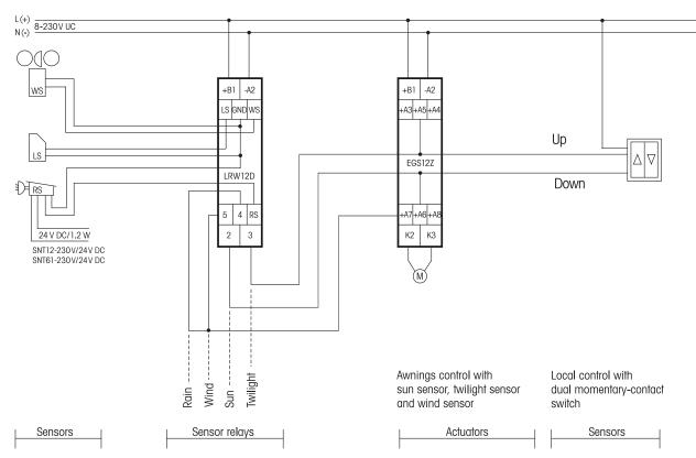
When controlling with 230 V (+B1= L, -A2=N) the 230 V awning motor is directly connected to K2, K3 and N. Otherwise a motor isolating relay MTR12-UC must be interconnected to K2/K3.
