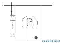
Newer rotary dimmers and rotary dimmers with phase cut control for electronic transformers cannot be used. The EUD61 universal dimmer and a button from the corresponding switch range can replace a pushbutton dimmer.
