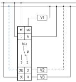
If (N) is connected, the zero passage switching is active.
