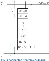
If N is connected, the zero passage switching is active.
