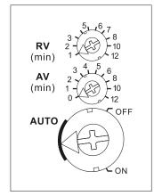
RV = release delay (delay time)
