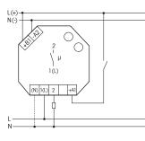
If N is connected, the zero passage switching is active.
