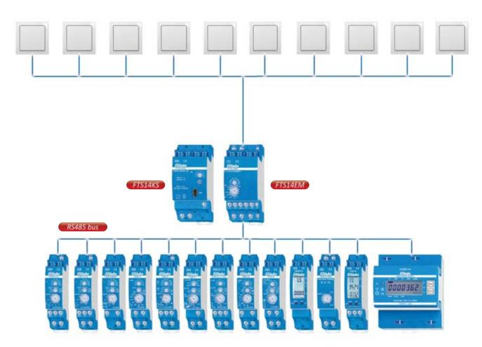
All optional possibilities can be combined as required: FTS14EM with actuators, the wireless antenna module FAM14, the pushbutton wireless output module FTS14FA and the pushbutton gateway FTS14TG for connection to pushbutton couplers FTS61BTK.
