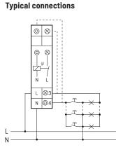
3-wire circuit, resettable.
