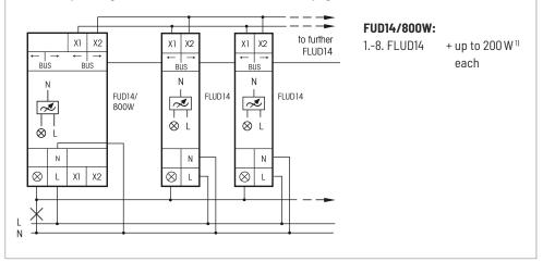
Capacity increase for additional lamps (추랴) in dimmer switch operating modes AUTO, LC4, LC5 and LC6. For operating modes EC1, 2 and LC1, 2, 3, see next page.
