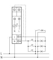
4-wire circuit with attic lighting, resettable.
